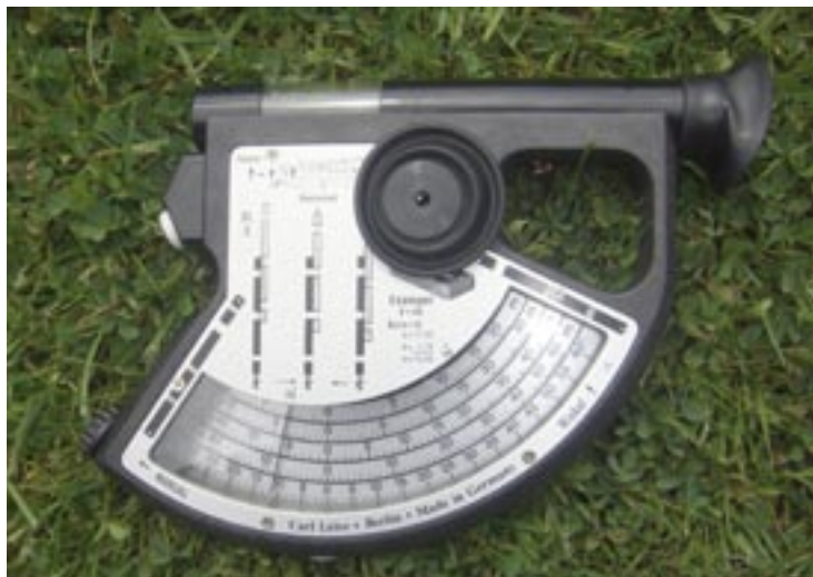
Figure 13. An hypsometer, used for measuring tree height
