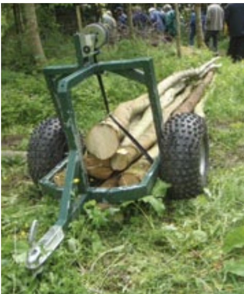
Figure 11. Extraction of broadleaf thinnings by quad using a skidder (left) or a trailer (right)
