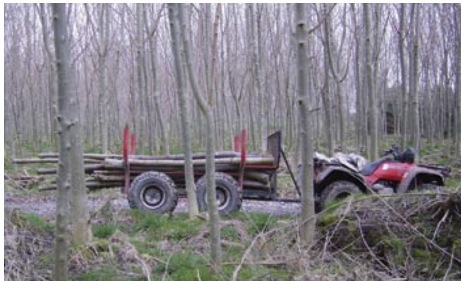
Figure 11. Extraction of broadleaf thinnings by quad using a skidder (left) or a trailer (right)
